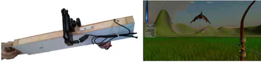
Figure 8: Heracles prototype. Left: bow with gyro. Right: screen view on mobile device.
